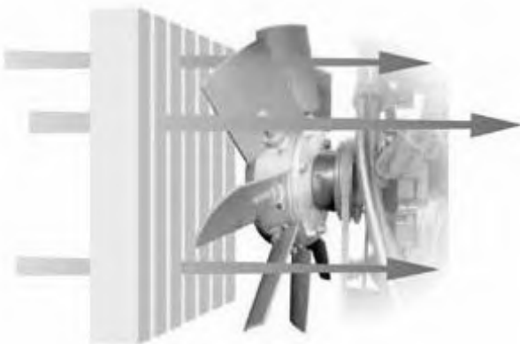
Airflow through radiator for cooling
