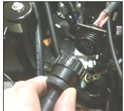
Location and identification of the emergency control unit connection point
