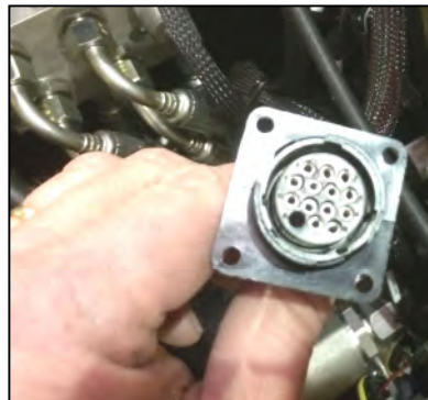
Location and identification of the emergency control unit connection point
