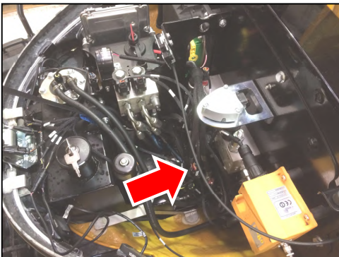
Location and identification of the emergency control unit connection point
