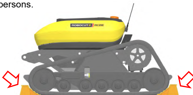
Chock machine front and rear when unattended or stored
