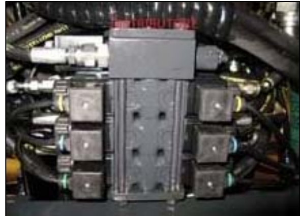
Hydraulic distributor valve
