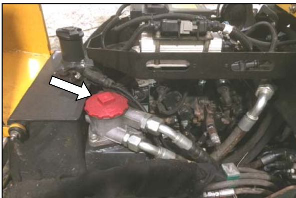
Hydraulic oil filter location
