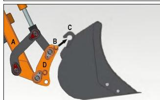
Ensure the handle for operating the quick-attach pins is in the vertical position (pins retracted).
