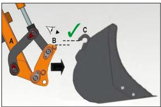
Operate lift arms (A) to position and locate upper attachment bar (B) in the bucket's top brackets (C); the angle of mechanism (D) may need to be adjusted on the controls to permit coupling.
