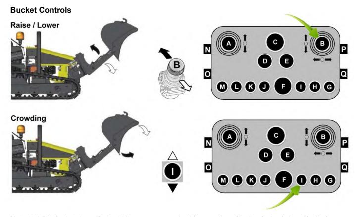
Note: TOE-TIP bucket shown for illustration purposes; controls for operation of the Loader bucket are identical.
