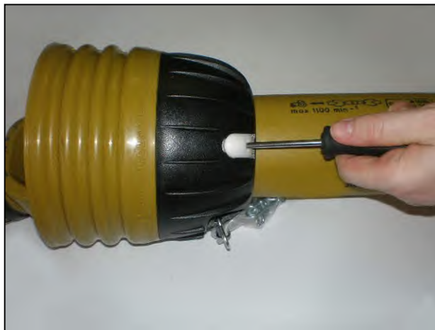
Insert screwdrivers into the clasps
