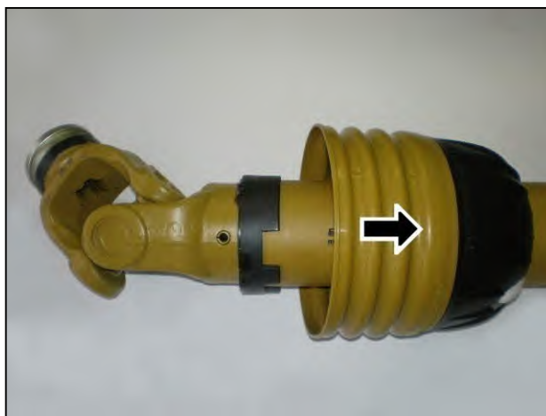
Slide shield back to reveal universal joint
