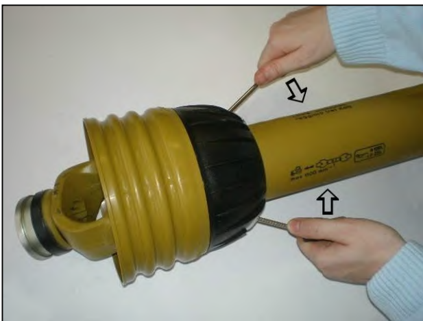
Pry clasps open to release the shield
