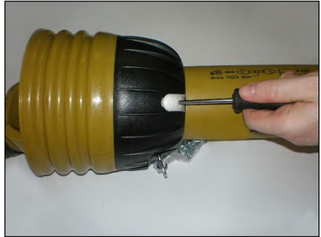
Insert screwdrivers into the clasps
