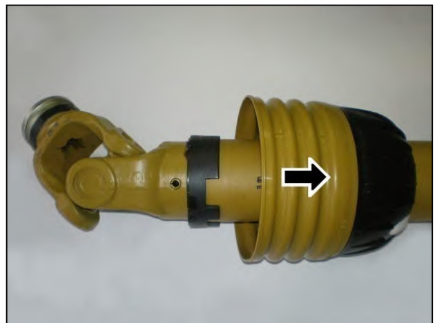
Slide shield back to reveal universal joint
