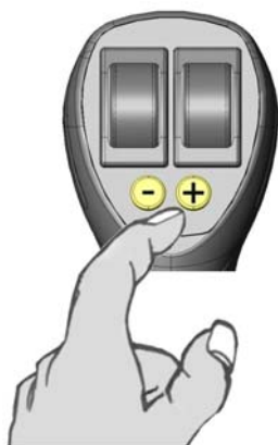
Advanced Lift Float; Pressure Adjustment
