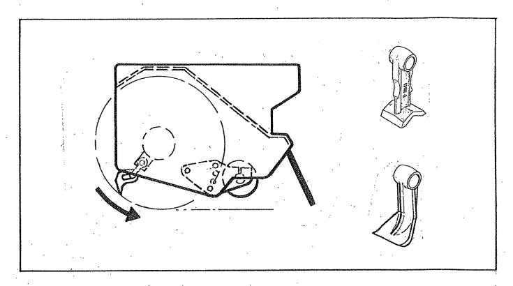
Where the size of the material to be cut makes it necessary for the front hood and carrier plates to be removed to allow the rotor to cut, the rotor must always cut with a downwards rotation.
