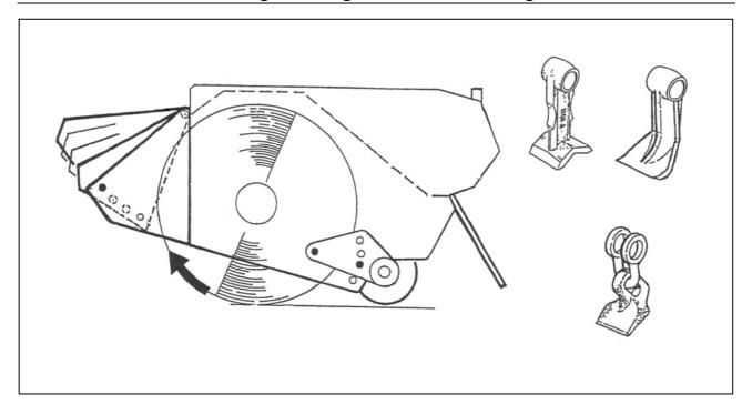
For the best finish the rotor should cut with 'upward' rota tion. The roller should be set slightly above the rotor - *i.e. in position 1.*
