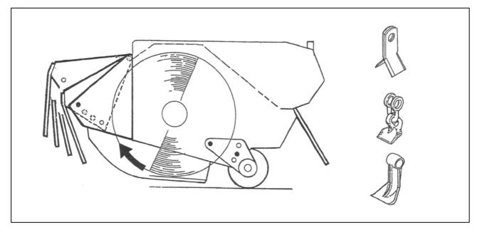
When mowing the rotor <u>must always</u> cut with 'upwards' rotation and the roller <u>must alway s</u> be set below the level of the skid (or the rotor if skids are not fitted) – *i.e.* positions 2 - 6. The front hood has four adjustment positions for height – *the lowest position that will allow* material into the flailhead to be cut should always be selected.
