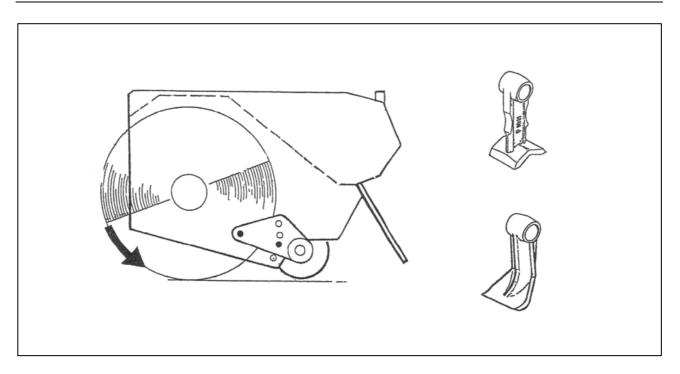
Where the size of the material to be cut makes it necessary for the front hood and carrier plates to be removed to allow the rotor to cut, the rotor must always be set to cut with 'downward' rotation – *this will result in a poorer finish and requires more power than 'upward' cutting.* The roller should be set slightly above the rotor - *i.e. in position 1.*
