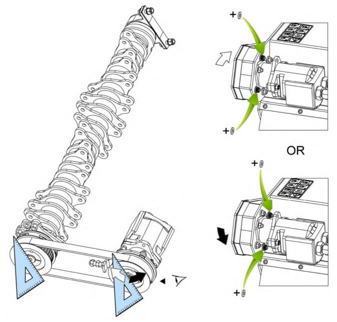
When pulleys have been correctly aligned the required adjusted to the correct tension; refer to belt adjustment section for details of belt tensioning procedure.
