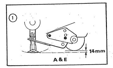
Positions 2,3,4,5, and 6 provide a selection of roller heights for mowing operations. The length of the finish required and the condition of the ground surface will determine the setting selected.
