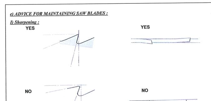
The saw teeth are sharpened very precisely to a shape that is in proportion to the angle of attack & the angle of clearance.
