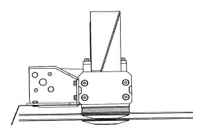
Saw blades must never be in direct contact with the wooden pallet or the floor otherwise you may bend them. (the protective rear cover does not eliminate possible distortion of the blade).
