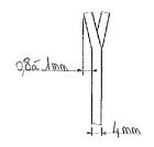
The blades diam.600, 650 and 700 having a body width of 4mm must have a set of between 0.8 and 1mm to each side.
