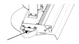
. The L.E.M. © cutter is fitted with a centralised lubrication system for the base unit. If an additional module has been fitted it will not have centralised lubrication to it's bearing. Lubricate as shown below.
