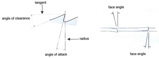
The recommended angle of attack must be set between  $5^{\circ}$  for cutting hard wood and  $10^{\circ}$  for cutting green wood.
