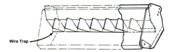
The flailhead is equipped with a 'wire cutting' edge welded into the underside – this plate should not be interfered with in any way. If wire becomes caught in the rotor the machine must be switched off immediately and the wire removed.
