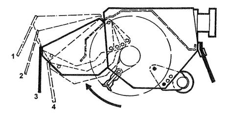
For mowing work the rotor must always cut with an upwards rotation and the roller set to a working height that is below the level of the skids *(or rotor if skids are not fitted)* – i.e. in position 2 or position 3 as shown on the previous page.
