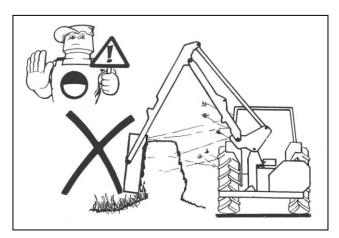
Cut the side and bottom of the field side first. This leaves the maximum thickness of hedge on the road side to prevent the possibility of debris being thrown through the hedge into the path of oncoming vehicles.
