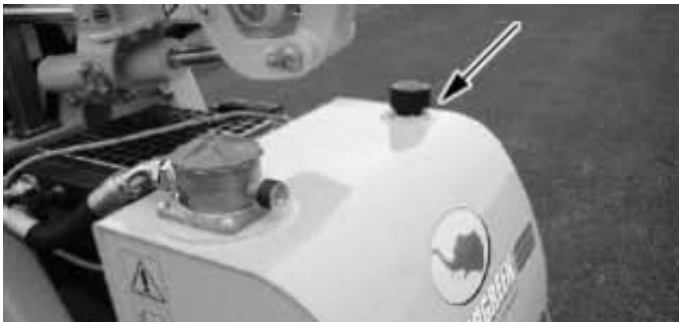
Hydraulic tank filler location
