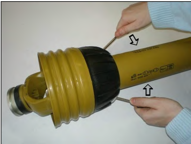
Pry clasps open to release the shield
