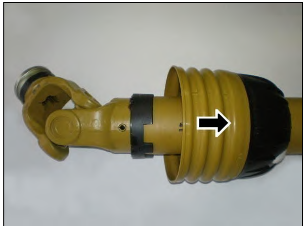
Slide shield back to reveal universal joint
