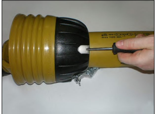
Insert screwdrivers into the clasps
