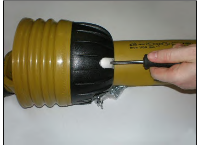
Insert screwdrivers into the clasps
