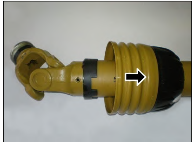
Slide shield back to reveal universal joint
