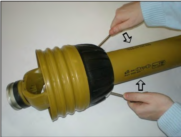
Prise clasps open to release the shield
