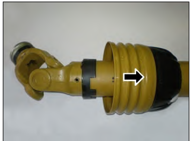
Slide shield back to reveal universal joint
