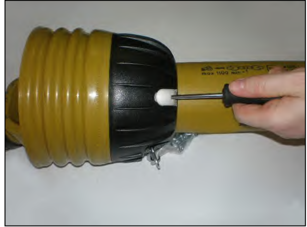
Insert screwdrivers into the clasp
