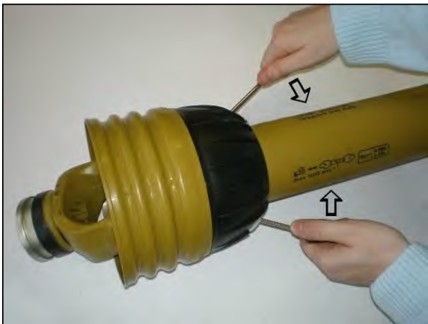
Pry clasp open to release the shield
