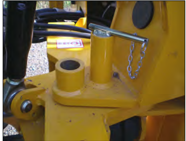
Slew Unlocked – only for working
