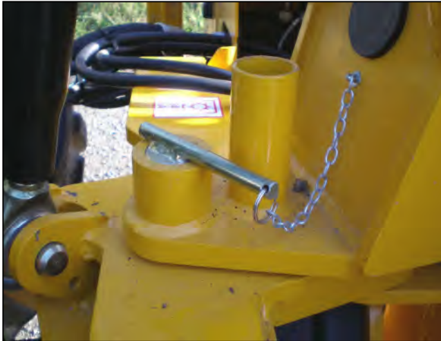
Slew Locked – always for transport & storage
