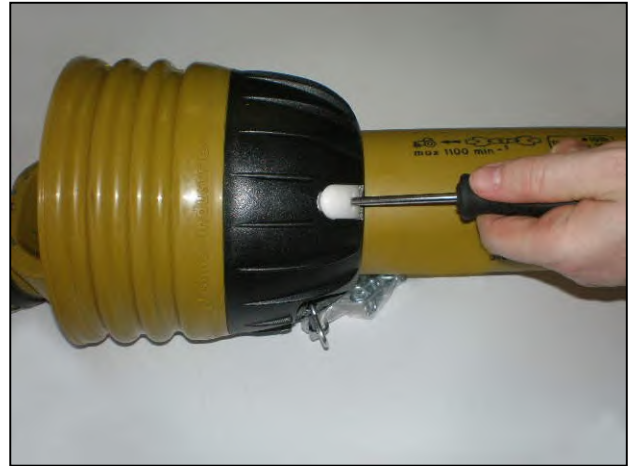
Insert screwdrivers into the clasps
