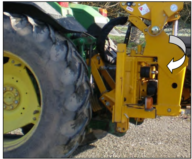
Open lift ram tap - slew machine to the side of tractor in work position.
