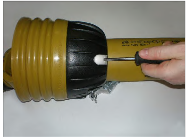
Insert screwdrivers into the clasps
