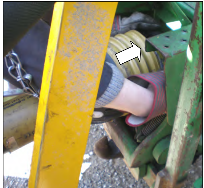
Attach PTO shaft to the output shaft of the tractor.
