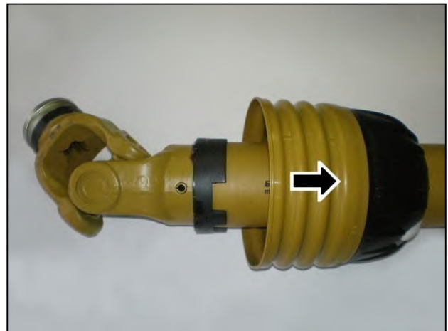
Slide shield back to reveal universal joint
