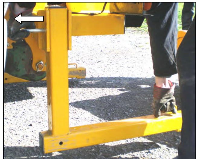
Axle models: remove legs and stow in mainframe. Linkage models: raise legs and secure with pins.
