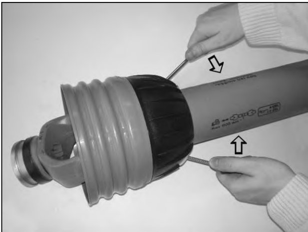
Prise clasps open to release the shield.
