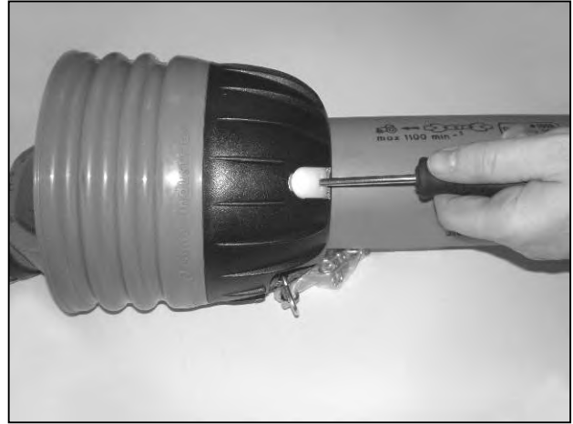
Insert screwdrivers into the clasps.
