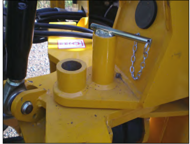
Slew Unlocked; only for working
