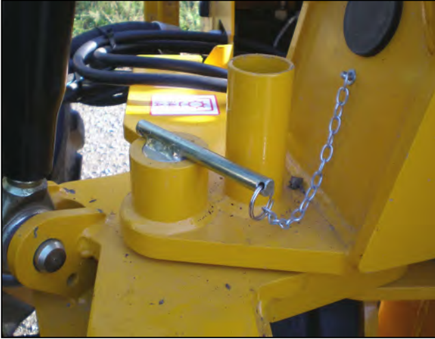
Slew Locked; always for transport & storage
