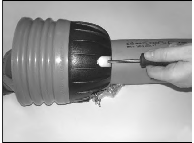
Insert screwdrivers into the clasps
