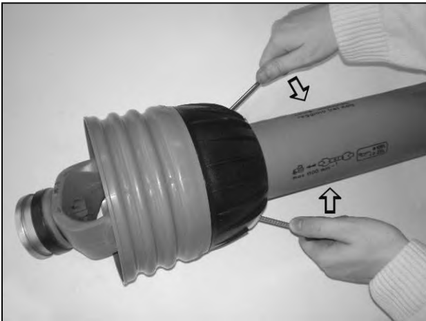
Prise clasps open to release the shield
