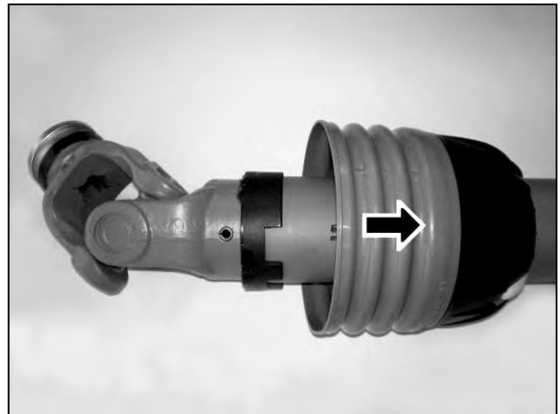
Slide shield back to reveal universal joint
