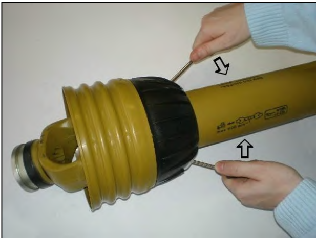
Prise clasps open to release the shield
