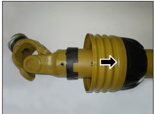
Slide shield back to reveal universal joint
