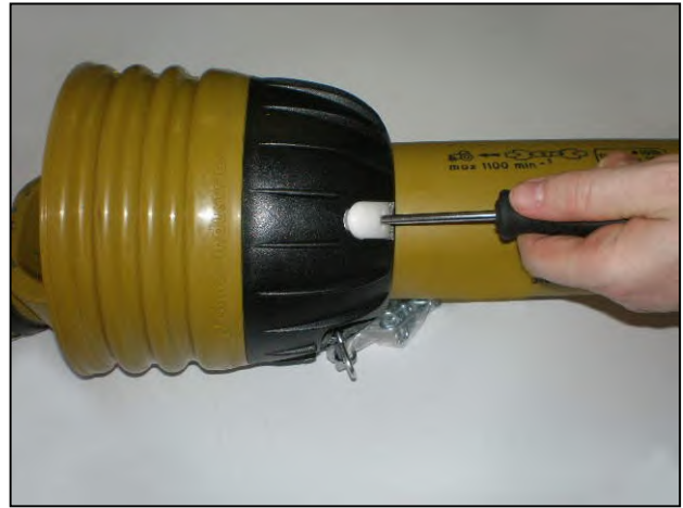
Insert screwdrivers into the clasps
