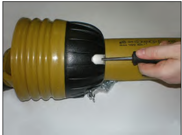
Insert screwdrivers into the clasps
