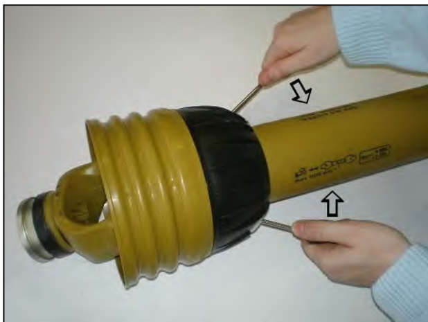
Pry clasps open to release the shield
