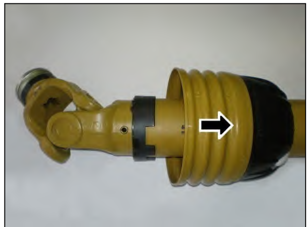
Slide shield back to reveal universal joint
