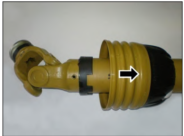
Slide shield back to reveal universal joint
