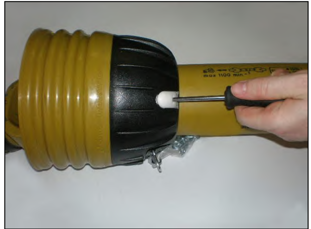
Insert screwdrivers into the clasps
