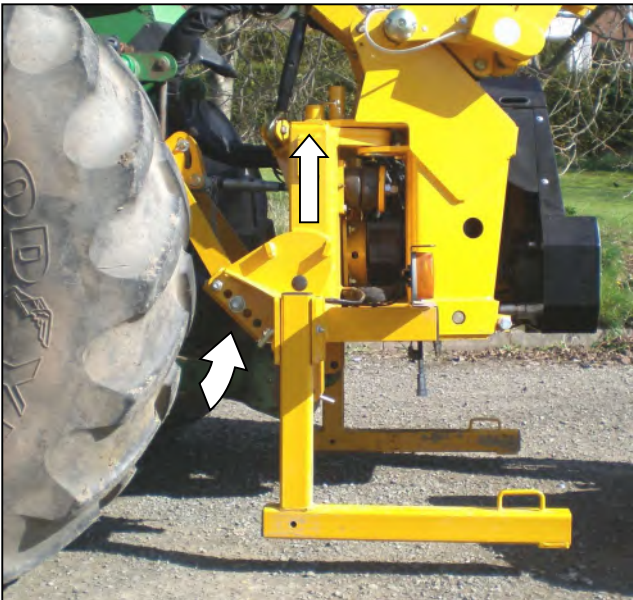
Tighten tractor stabilisers - raise tractor linkage to lift the machine to its working height.
