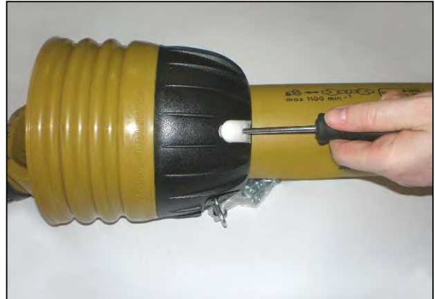
Insert screwdrivers into the clasps
