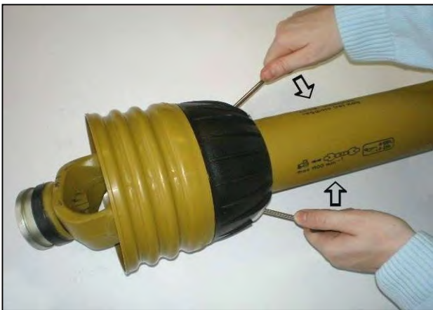
Pry clasps open to release the shield
