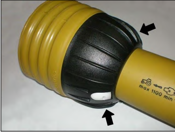
Shaft shield fixing clasps
