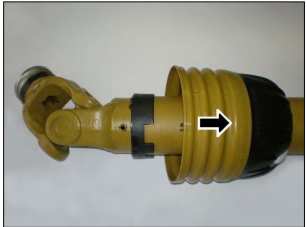
Slide shield back to reveal universal joint
