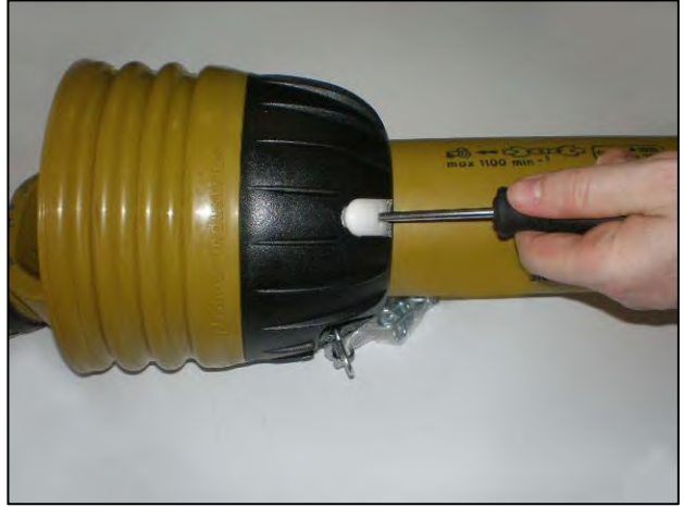
Insert screwdrivers into the clasps
