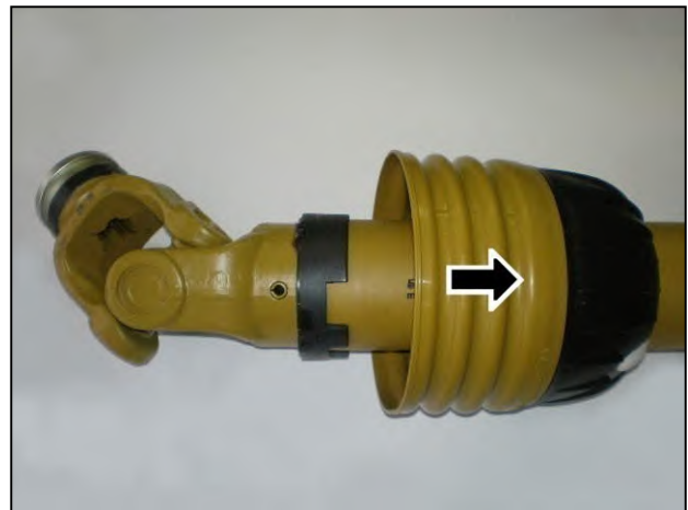
Slide shield back to reveal universal joint
