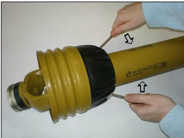
Prise clasps open to release the shield
