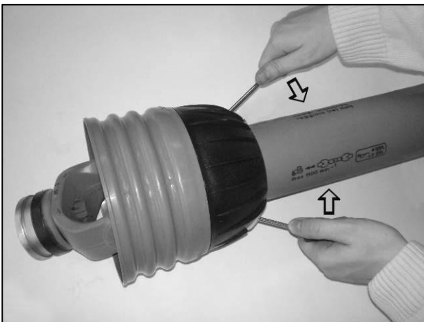
Prise clasps open to release the shield
