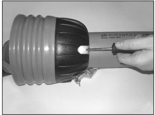
Insert screwdrivers into the clasps
