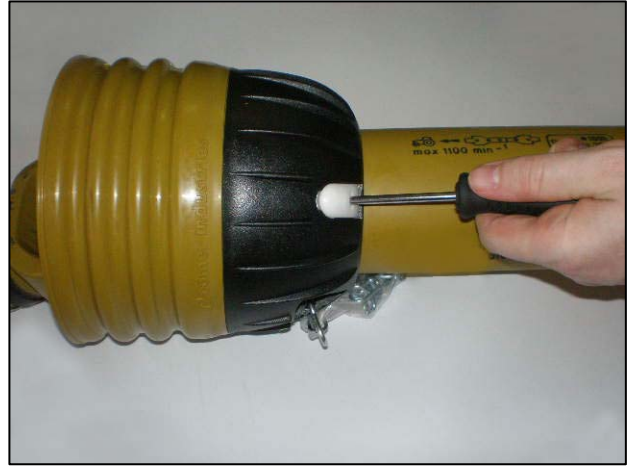
Insert screwdrivers into the clasps
