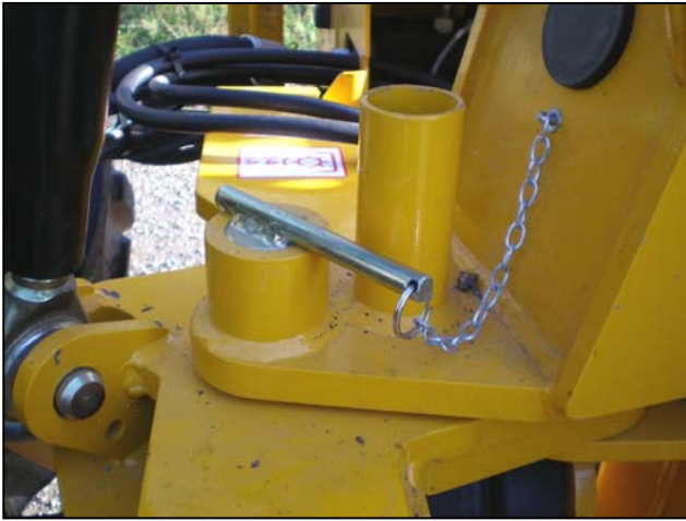
Slew Locked – always for transport & storage
