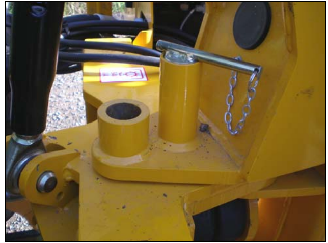
Slew Unlocked – only for working
