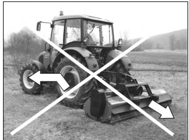
Raise the machine before turning or reversing.
