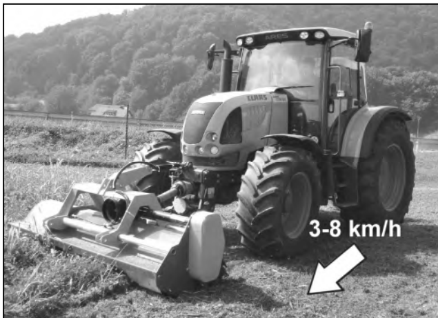
Optimal forward working speed 3-8 km/h.
