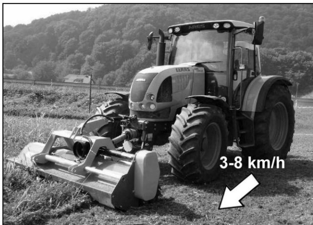
Optimal forward working speed 3-8 km/h
