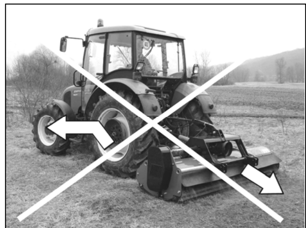
Raise the machine before turning or reversing
