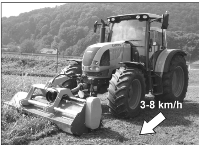
Optimal forward working speed 3-8 km/h
