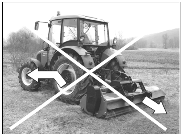
Raise the machine before turning or reversing
