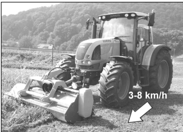
Optimal forward working speed 3-8 km/h
