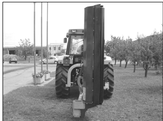
190 & 225 Models are transported vertically
