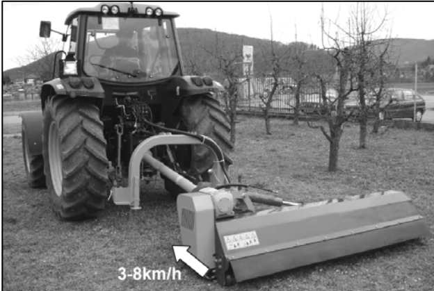
Optimal forward working speed 3-8 km/h
