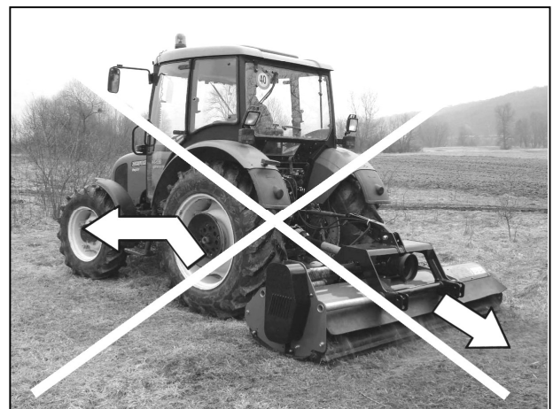
Raise the machine before turning or reversing
