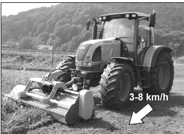
Optimal forward working speed 3-8 km/h
