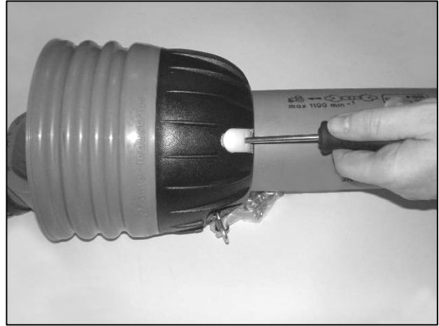
Insert screwdrivers into the clasps
