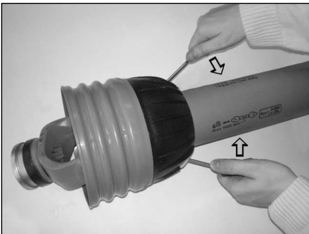
Pry clasps open to release the shield
