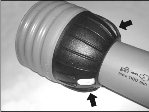
Shaft shield fixing clasps
