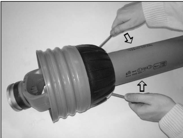
Pry clasps open to release the shield
