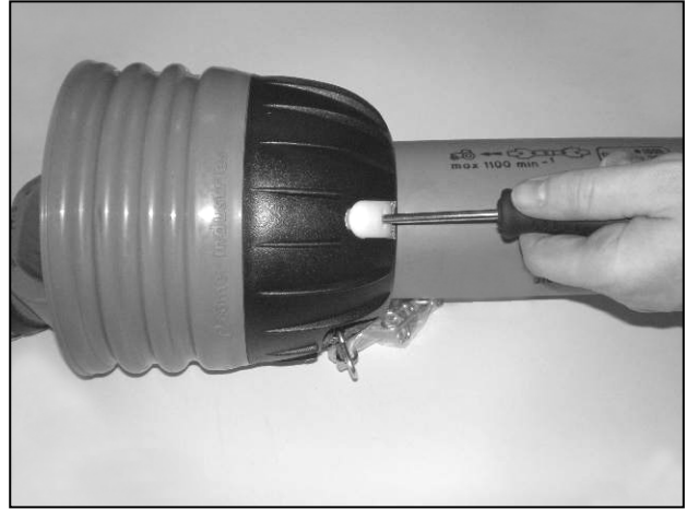
Insert screwdrivers into the clasps
