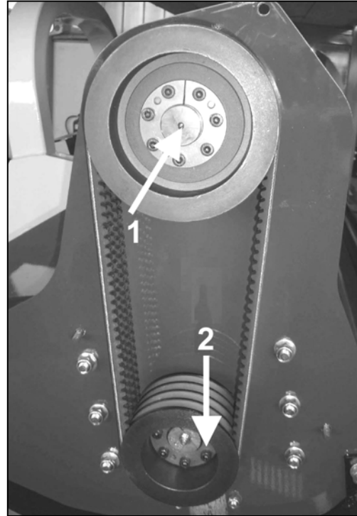
Taper Locks – check tightness on new machines after initial 2 hours of work
