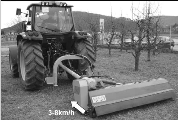
Optimal forward working speed 3-8 km/h
