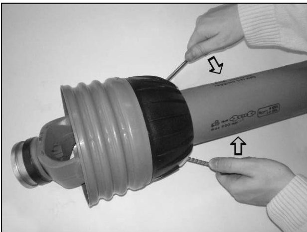
Pry clasps open to release the shield
