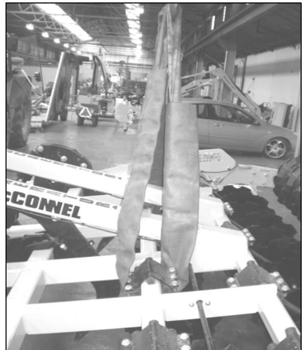
It is vital that all lifts are performed vertically as any sideways pull tends to overload the edges of the belt with potential risk of either tearing them or moving them over possible rough edges that risk cutting them.
