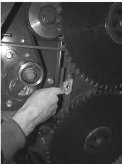
Set tension of the centre belt
