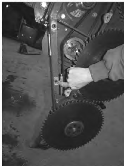
Set tension of lower belt
