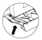
**Protection Guard** - Remove only with the motor switched off and the oil NOT under pressure.
