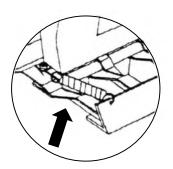
Protection Guard - Remove only with the motor switched off and the oil NOT under pressure.
