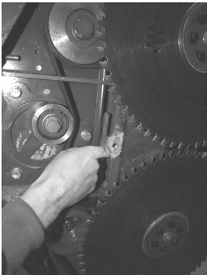
Set tension of the centre belt
