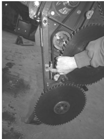
Set tension of lower belt
