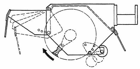
For normal trimming work on hedges the roto r should be set to cut with an upwards rotation – this produces a better finish to the work and demands lower power requirement. Front hood and rear flap must always be in position.
